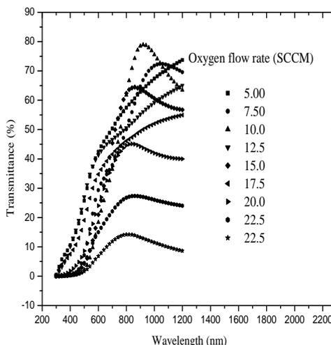
**Figure 3.1:** Variation of transmittance (%) with Oxygen flow rate
