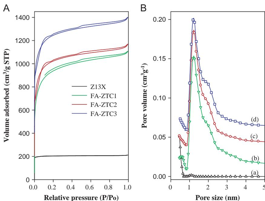
**Fig. 3** Nitrogen sorption isotherms (A) and pore size distribution curves (B) for (a) zeolite 13X, (b) FA-ZTC1, (c) FA-ZTC2 and (d) FA-ZTC3. For clarity, sorption isotherms of FA-ZTC2 and FA-ZTC3 are offset (y-axis) by 200  $\text{cm}^3/\text{g}$  and 400  $\text{cm}^3/\text{g}$  respectively, and the PSD curves (b), (c) and (d) are offset (y-axis) by 0.01, 0.04 and 0.06  $\text{cm}^3/\text{g}$  respectively.
