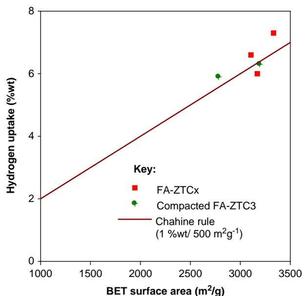
**Fig. 9** Correlation between surface area and hydrogen uptake capacity for FA-ZTC samples.
