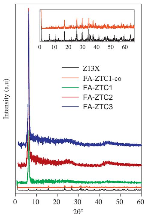
**Fig. 1** Powder XRD patterns of zeolite templated carbons (FA-ZTC1, FA-ZTC2 and FA-ZTC3) prepared at variable heating ramp rate (5, 10 and 15 °C/min respectively). Patterns for the zeolite/carbon composite (FA-ZTC1-co) and zeolite 13X (Z13X) are also shown.
