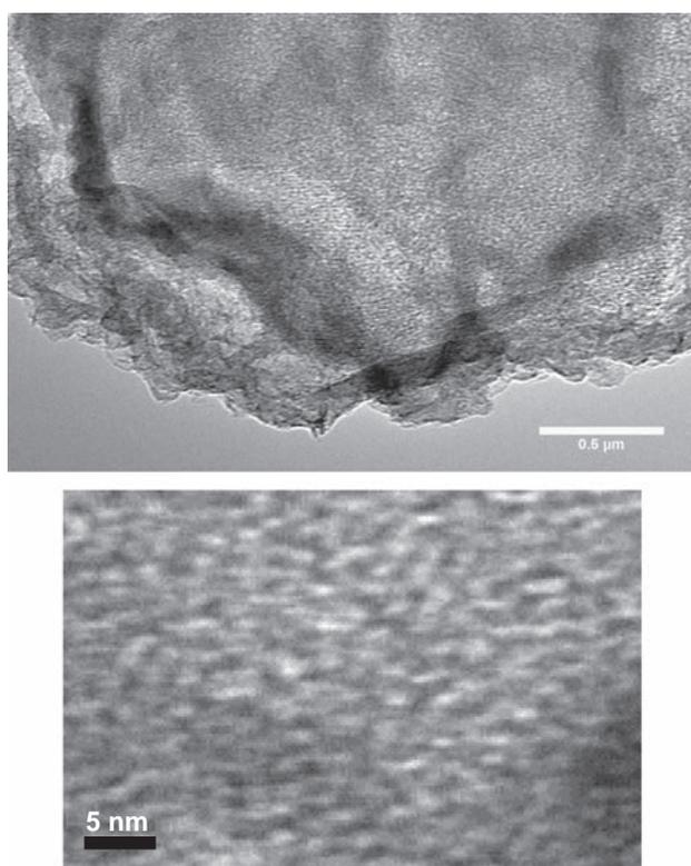
**Fig. 4** TEM images of zeolite templated carbon (sample FA-ZTC2).
