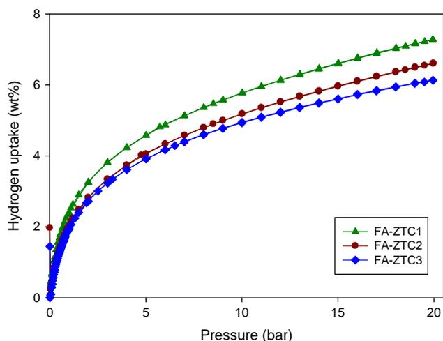
**Fig. 7** Hydrogen uptake isotherms of zeolite templated carbons at 77 K.
