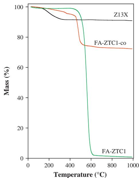
**Fig. 2** TGA curves for zeolite 13X (Z13X), zeolite/carbon composite (FA-ZTC1-co) and zeolite template carbon (FA-ZTC1).
