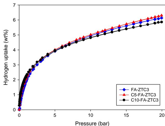
**Fig. 8** Hydrogen uptake isotherms at 77 K of zeolite templated carbon (FA-ZTC3) before and after compaction at 5t (C5-FA-ZTC3) and 10t (C10-FA-ZTC3).
