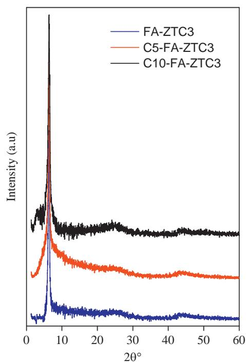
**Fig. 5** Powder XRD patterns of zeolite templated carbon (FA-ZTC3) before and after compaction at 5t (C5-FA-ZTC3) and 10t (C10-FA-ZTC3).
