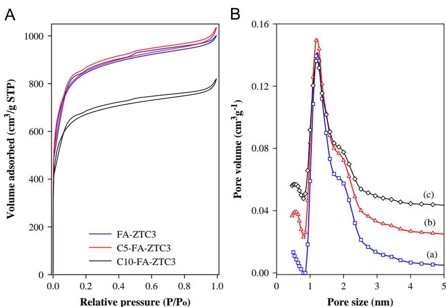
**Fig. 6** (A) Nitrogen sorption isotherms and (B) corresponding pore size distribution curves of zeolite templated carbon (FA-ZTC3) before and after compaction at  $5t$  (C5-FA-ZTC3) and  $10t$  (C10-FA-ZTC3).
